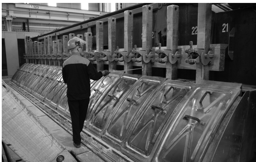
Figure 5. A small part of the pot line in the Alcoa aluminum smelter at Fjarðaál, Iceland. 2008 photograph. Image used courtesy of Alcoa Inc.
